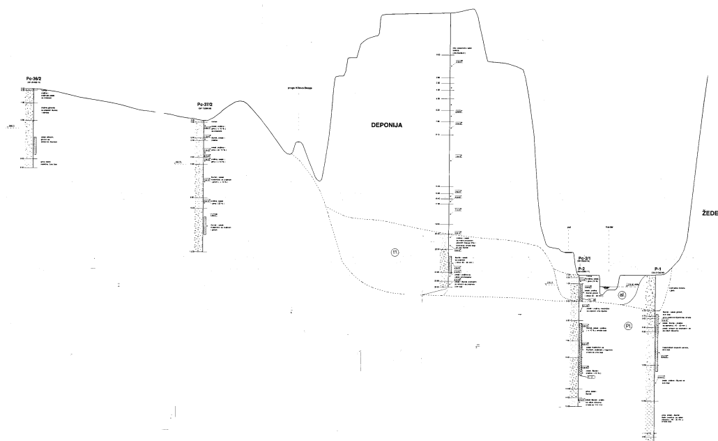
Figure 27_ density of the dumpsite layers according to Cerni core drill study
